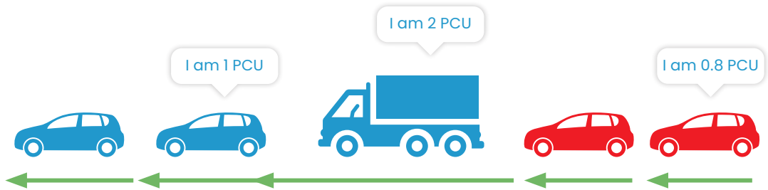
Figure 4: Example of different PCU values per type of vehicle (@University of Stuttgart)
